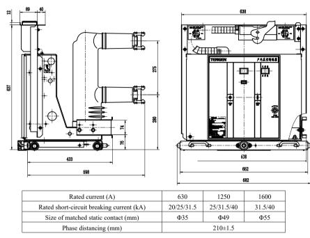
Note: The meshing size of dynamic and static contacts is not less than 15mm.
